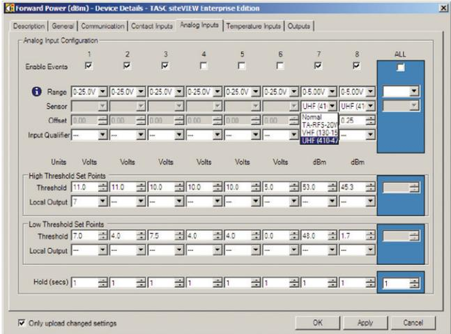
It is important to know the strength of the radio signal in order to make sure the system is ready to perform when called upon. The BPS from TASC will be able to inform you if the antenna has been compromised by reporting back an alarm. Armed with this information, the appropriate action can be taken to remedy the problem.
