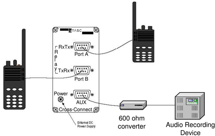
**Figure 5 Cross-Connect Connections**
