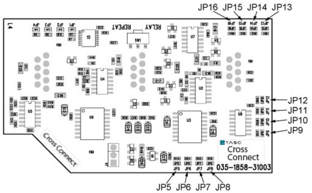
Figure 8 Lockout Jumper Locations
