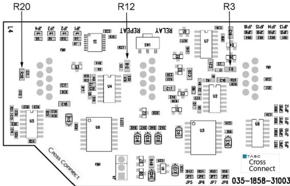
Figure 6 RX Input Impedance Resistors
