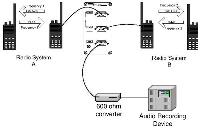
**Figure 2 Relay Operation**
