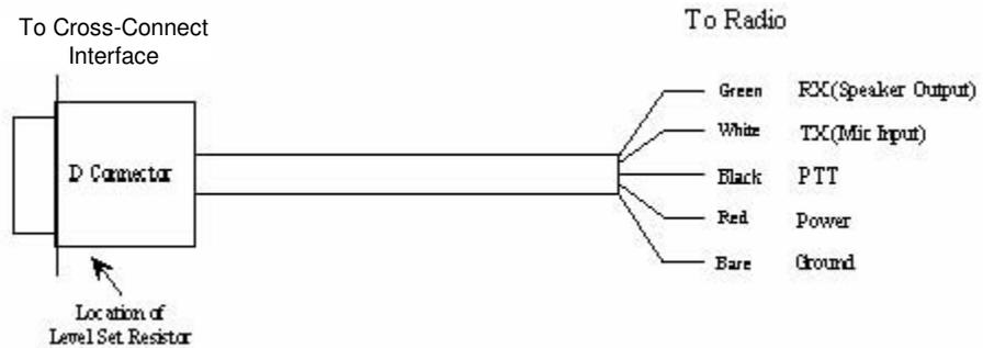
**Figure 3 Cross-Connect Cable**
