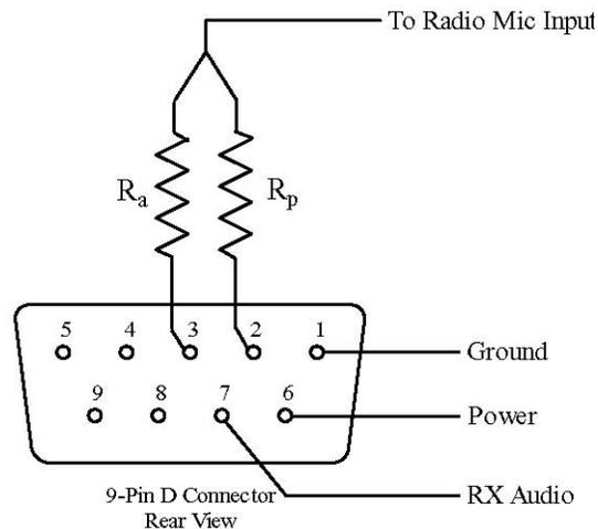
**Figure 7 Setup for Shared Mic & PTT Line**
