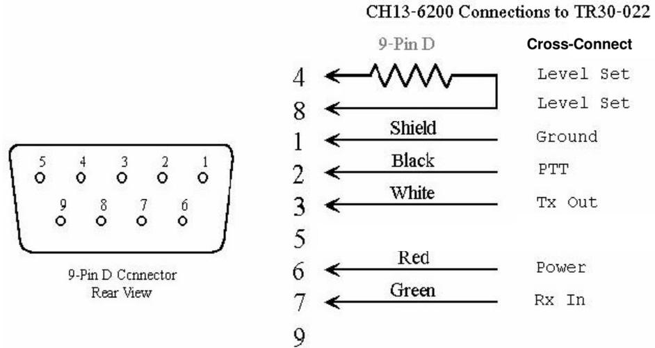
**Figure 4 9-Pin D-Sub Connection**
