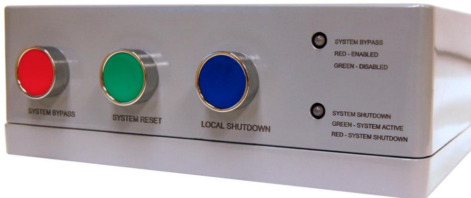
Figure 3: Front image of Industrial Controller
