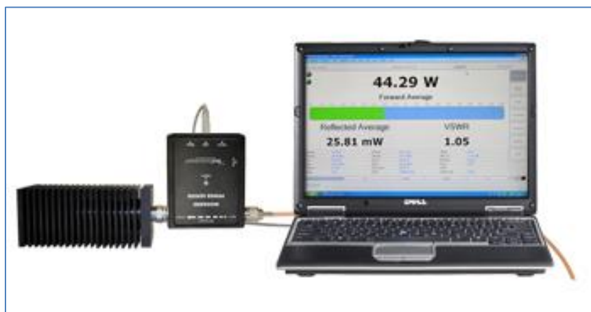
Figure 10 - Example of a Power Sensor (Measuring Forward Power) 14
